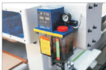
Automatic lubricate setting
