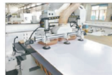
Strong adsorption automatic feeding sucker
