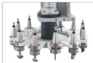
Hammer-type changing tool system
