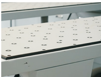
chrome plated surface to avoid board scratching
