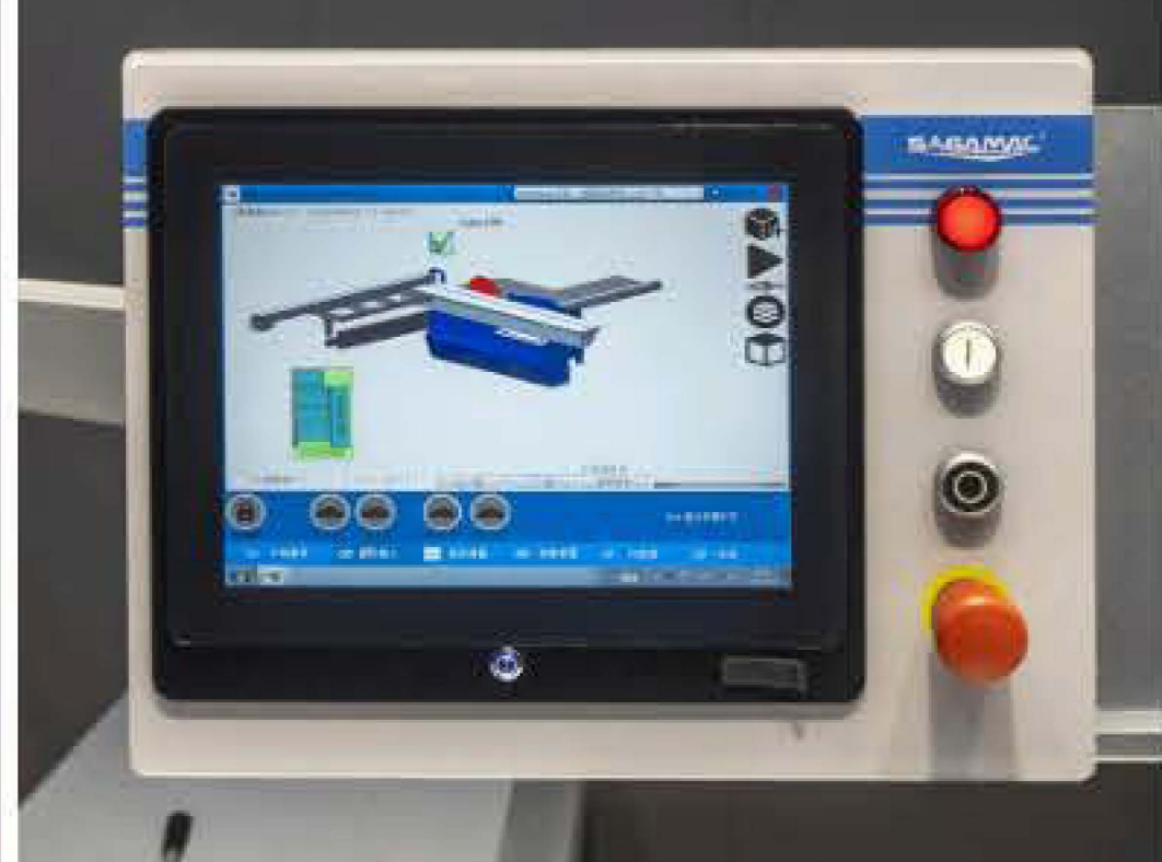
Electrical tilting of blade can be LCD screen to indicate or fully automatic set on control panel
