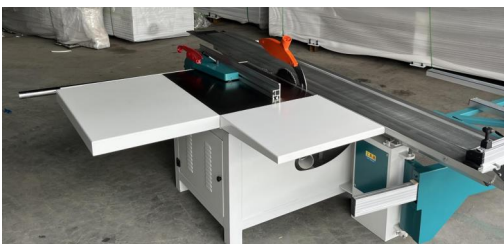
7. The crosscut fence can be attached to the sliding table without the use of tools. The end stop provides you with the exact 90° position.
