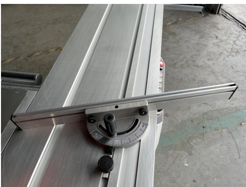
6. The solid outrigger makes it possible to process large and heavy workpieces
